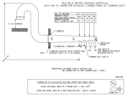
NOTE A: OPENING MUST BE TWO (2) INCHES LARGER THAN DUCT (ALL THE WAY AROUND). THE DUCT MUST BE CENTERED WITHIN THIS OPENING.
